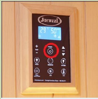
Go to your sauna and with it turned off, press and hold the Power button for about 7 seconds until you hear a beep confirming that it is now in wireless setup mode.
