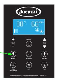
2. Lock Keypad - Light Button Will Continue To Work: Hold down the "OUTSIDE" button for 15 seconds. This will lock the entire keypad except the light button. To unlock the keypad, repeat the above step.
