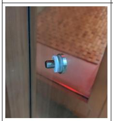
Best way to proceed from here is to place your bolts back into the holes with one washer on the outside and one on the inside.
