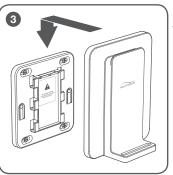
Attach the wall mount cover to the bracket
