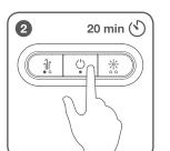
To turn on the  ${\sf HALO}{\sf ONE}^{\sf m},$  press and hold the POWER button for 2 seconds.
