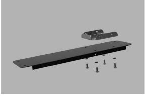
Install tower attachment plate using the 4 1/4-20 washer head screws and plastic washers, Using the 5/32 hex wrench.
