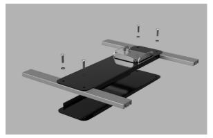
Take both top and bottom base plates and fit them together with the sides of the top plate overlapping the side of the bottom. Insert both legs making sure holes line up perfectly, then secure using 1/4-20 button head & large hole medium washers.
