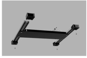
Install the 4 rubber feet on legs and side base plate using the 10-24 button head screws with a 7/64 hex wrench. Along with washer for side base screws.
